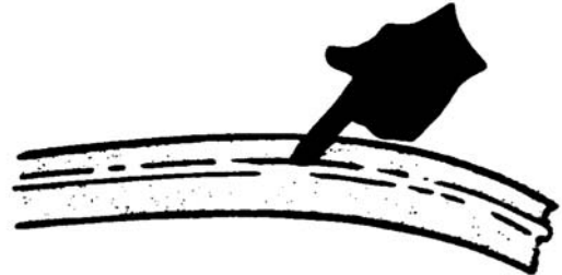
Figure 4-3. Belt Wear Due to Misalignment or Worn Pulley Groove
