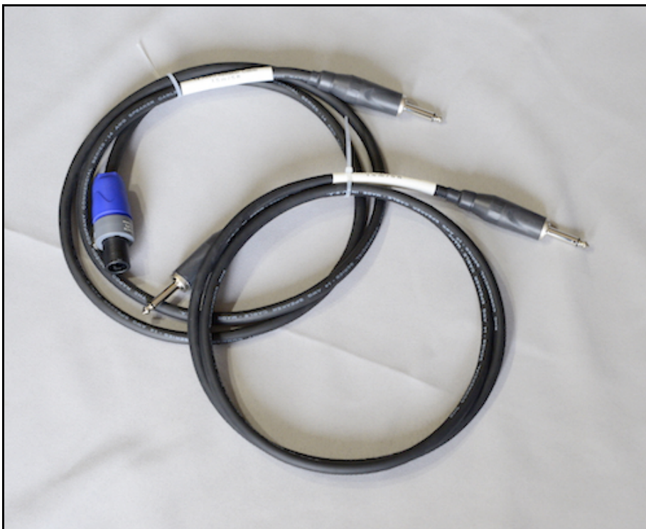
Speaker cables: Amphenol 1/4" TS both ends, Amphenol 1/4" TS with Neutrik Speakon 2-pole connectors.
