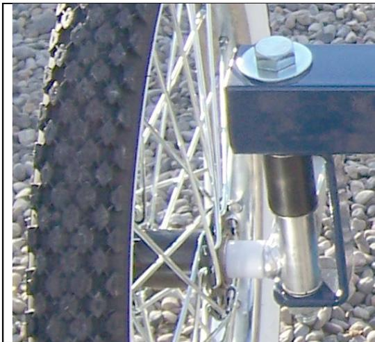
The kingpin bolt as it passes through the frame, the rubber damper and the spindle. Visible at the bottom of the spindle is a white ring of plastic.
