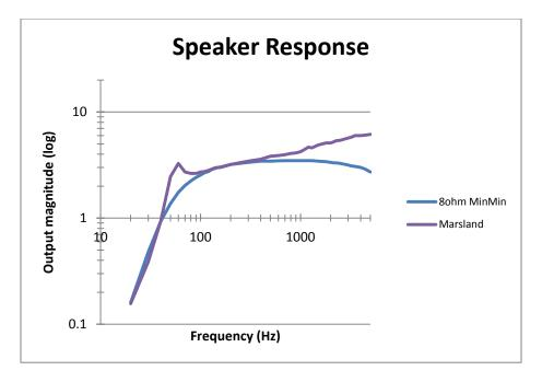
The difference in the voltage output represents the influence of the speaker. In this case, we can see that the speaker causes a natural increase in lower frequency response – as well as an increase in upper treble response.
