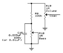
For a 'minimum' bass setting (full counter-clock-wise on the knob), the potentiometer is such that capacitor C15 is shorted to ground, with the effective circuit appearing as:
