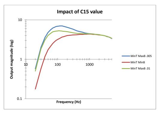
As the capacitance value gets smaller, the peak occurs at a higher frequency, and the the bass response increases.
