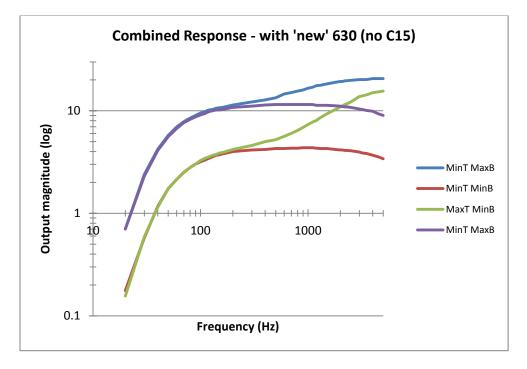
With C15 missing, the bass control does not selectively impact bass – but it still may be useful for some users in that it would allow the amplifier to overdrive more easily (since the levels are all pushed higher). Whether or not this is desired would depend on a particular user's taste.
